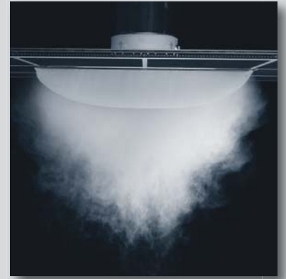
Cover: Smoke testing reveals uniform air flow pattern of a Surround Flow All-Fabric D-Fuser (500 CFM).
